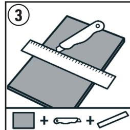
**Cut and install SoundStop® Underlayment** panels to fit size of room.
