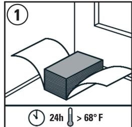
**Acclimate SoundStop® Underlayment** in installation area for 24 hours at room temperature, above 68°.
