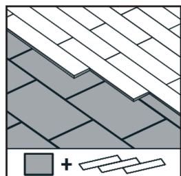
Stagger all laminate floor material seams. Do not line up with SoundStop® Underlayment seams.
