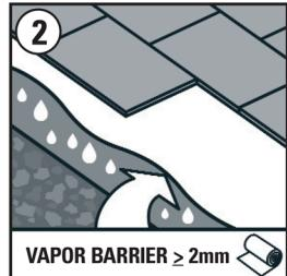
**Install a 2 mm or greater vapor barrier** over mineral based subfloor (e.g. concrete).
