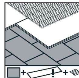
Adhere second subflooring, avoiding shared seams with SoundStop® Underlayment seams. Stagger all parquet or hardwood materials seams, avoiding shared seams with second layer of subflooring.
