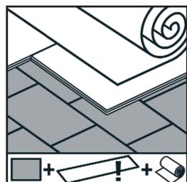
Adhere second subflooring, avoiding shared seams with SoundStop® Underlayment seams. Roll laminate floor material, avoiding shared seams with second layer of subflooring.
